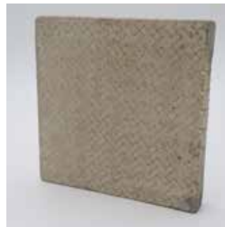
Concrete panels with embedded auxetic meshes to investigate the behaviour of the structural element.
