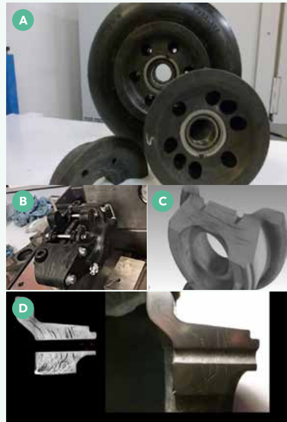
Examples of Thick section composite mouldings produced at Exeter. A) composite wheel hubs, these designed for the AgustaWestland AW139 helicopter, B) A composite automotive brake calliper mounted on Exeter's test rig ready for evaluation. C) CT Scan of an early wheel hub prototype- the dark lines are internal voids. The hub section and corresponding CT scan is shown on image D.
