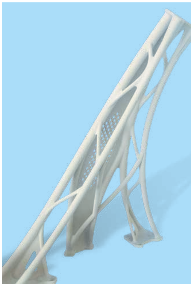
Topologically optimised demonstrator bracket made of experimental Victrex PAEK material. Design owned by 3T RPD Ltd., who reserves all rights to it.
