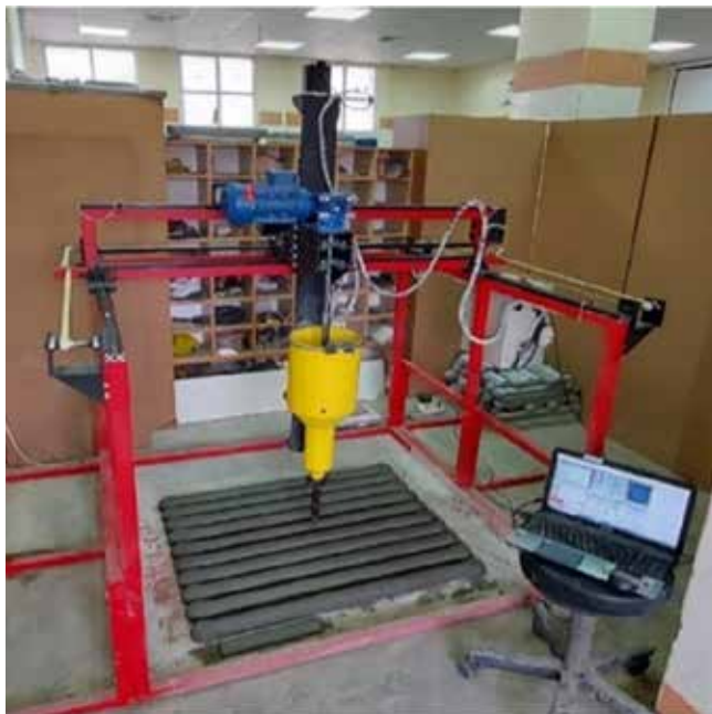
Laboratory Scale Concrete 3D Printer Developed by Our Team.
